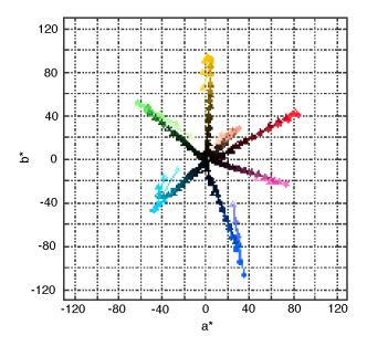
Figure 2. Hue shifts for the RIMM/ROMM RGB color encoding resulting from a typical nonlinear rendering transform.
