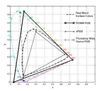
Figure 1. Comparison of primaries in x-y chromaticity coordinates
